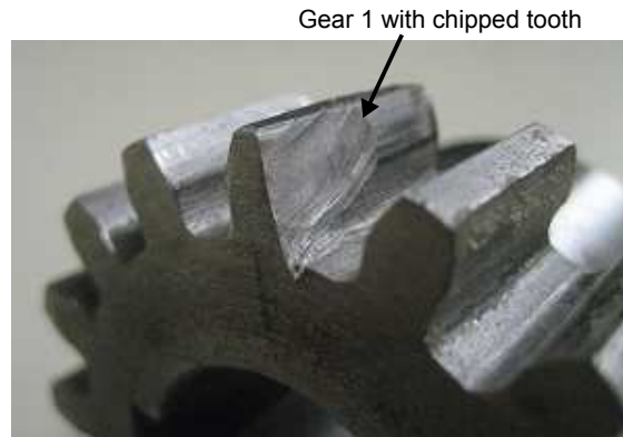
Figure 8: Faulty gear 1 with seeded tooth chip.
